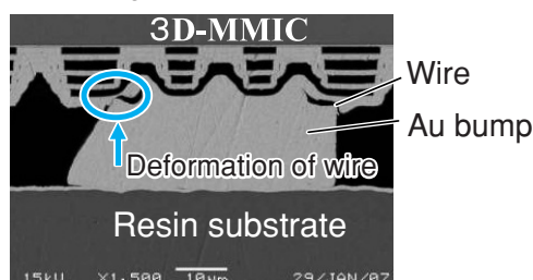
Fig.4 Example of Wiring Pattern Deformation
