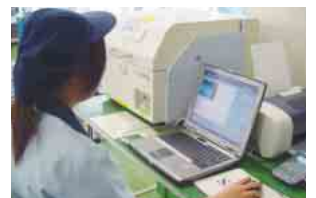
Monitoring toxic substances with a fluorescent X-ray spectroscopic analyzer
