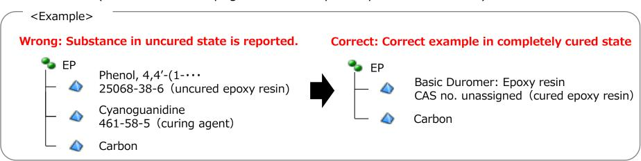
The followings show the correspondence between uncured and cured epoxy resins. Some uncured epoxy resins cure alone, but those having only two epoxy groups (O part) attached per molecule cannot cure\* alone because they cannot form a network structure geometrically.
