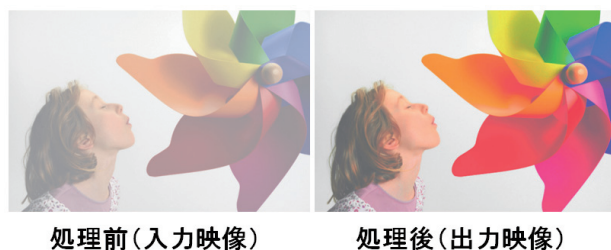
図5 直射日光補正処理の補正例 Fig.5 Example of Image Correction Processing in Direct Sunlight
