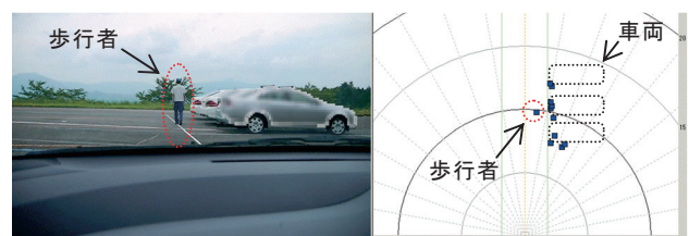
Fig.8 Outline of Detection Test of Pedestrian Walking around Vehicles
