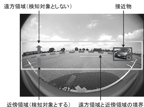
図11 近傍移動物と遠方移動物の分離手法 Fig.11 Separation Method of Objects Moving Nearby from ones in the Distance
