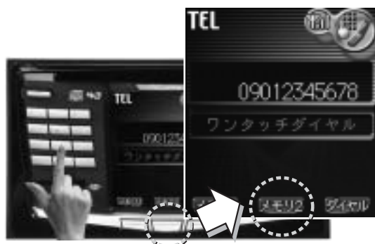
図-7 3-Functionボタン操作例 Fig.7 3-Function Button Control
