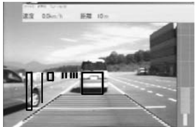
図-14 認識結果1 (割り込み) Fig.14 Recognition results 1 (vehicle cut-in)
