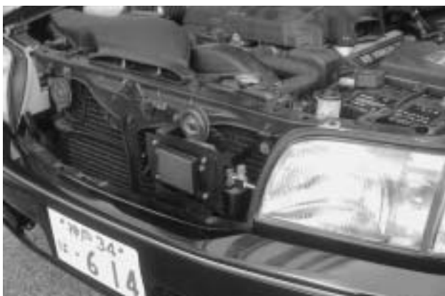
図-16 ミリ波レーダ取付け部 Fig.16 Millimeter-wave radar attachment
