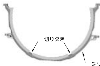
図-10 一次対策案の部品形状（裏側） Fig. 10 Component shape (back side) proposed in preliminary improvement plan
