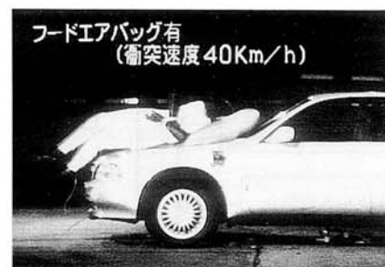
図-12 フードエアバッグと歩行者の関係 Fig.12 Relation of food airbag and pedestrian
