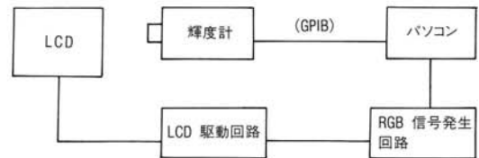
図-13 色度範囲測定システムの構成 Fig.13 Measuring system for range of chromaticity
