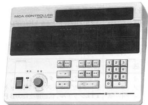
図-11 CCA-982A 指令局制御器外観図 Fig. 11 Exterior view of CCA-982A.
