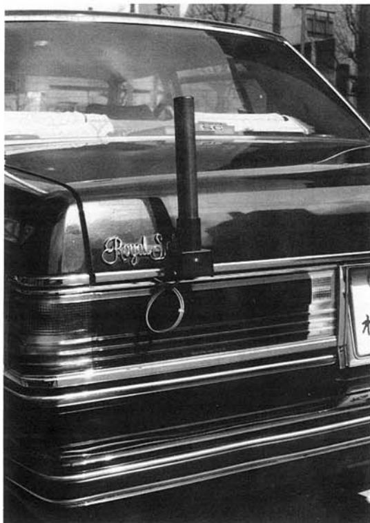
図-18 車載アンテナ Fig. 18 Antenna mounted on vehicle.
