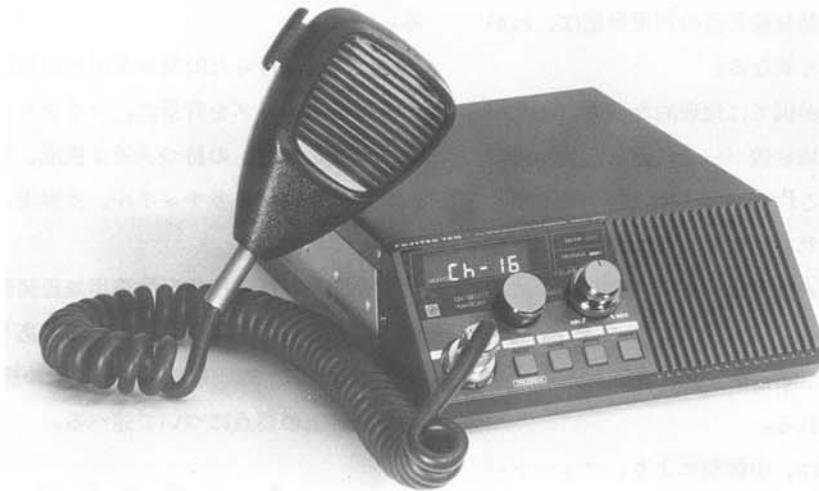
図-2 FTM15-3092/FTM40-3092型無線機外觀図 Fig. 2 Exterior view of FTM15-3092/FTM40-3092.
