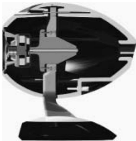
図-8 TD 512の内部構造 Fig.8 Internal structure of TD 512
