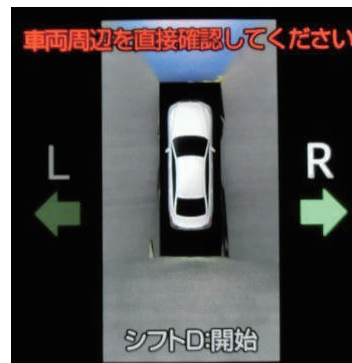
Fig. 8 Parallel departure HMI
