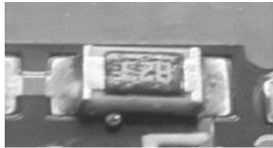
Fig. 6 Example of Solder Balls
