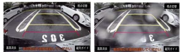
Fig. 1 Image Captured by Camera Having Lens with Water Drop
