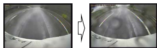
Fig. 2 Water Drop Attachment during Driving
