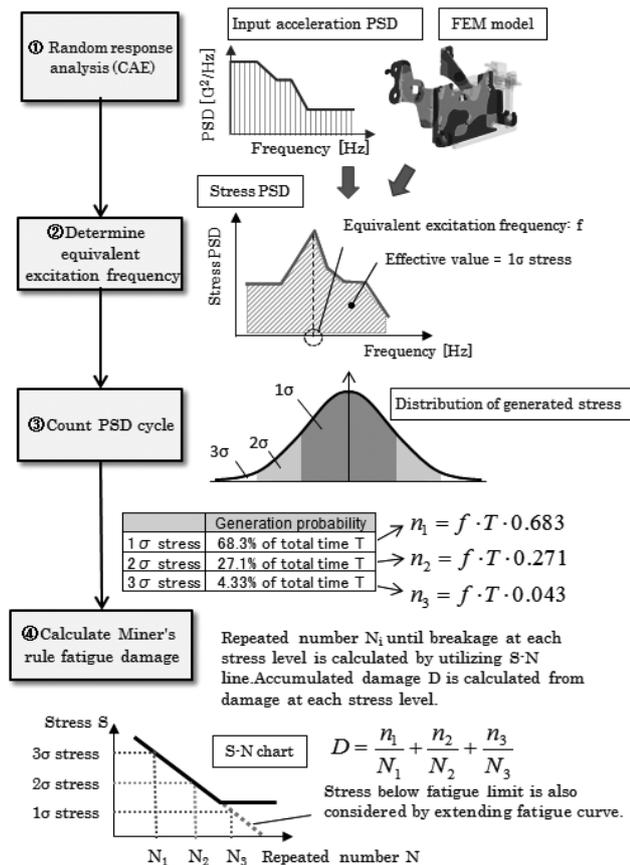
Fig.5 Calculation Procedure for Random Vibration Strength
