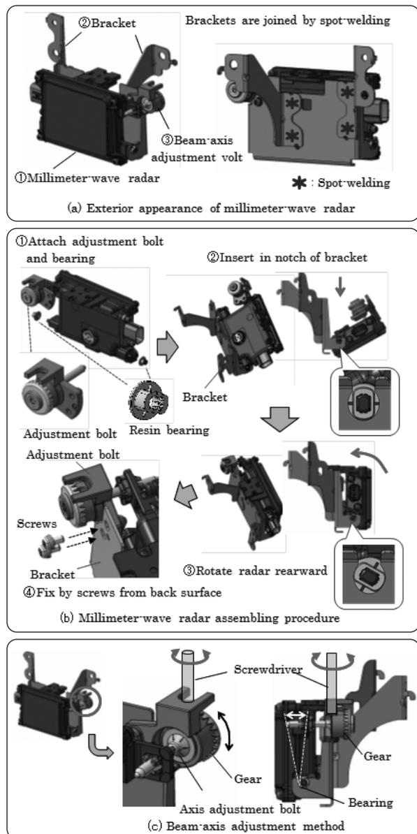
Fig.1 Structural of Bracket for Millimeter-wave Radar
