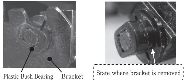
Fig.3 Abrasive Wear of Resin Bearing
