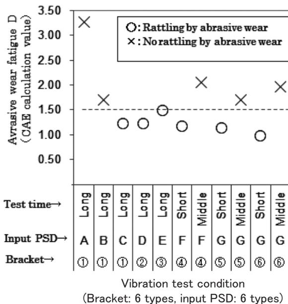
Fig.7 Comparison of Estimated Abrasive Wear Damage with Result of Real Machine Test
