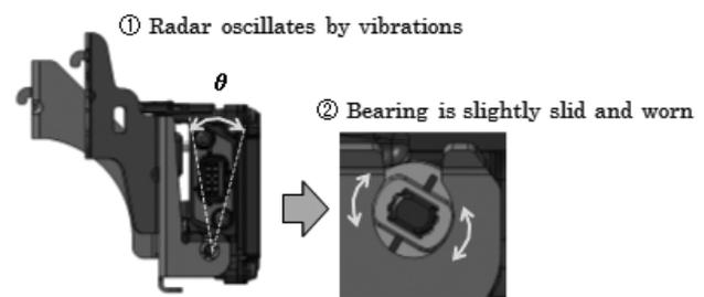
Fig.6 Mechanism of Abrasive Wear
