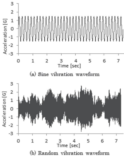
Fig.2 Sine Vibration and Random Vibration
