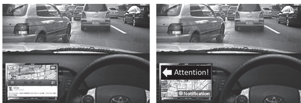
Fig.3 Example of HMI Control by DDC (Left: without HMI Control Right: with HMI Control)
