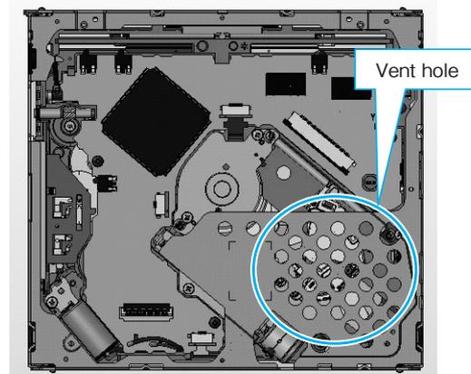
Fig.7 Heat Release Hole of Deck Chassis
