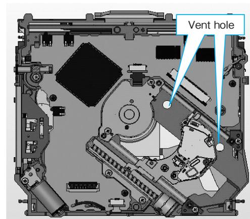
Fig.8 Heat Release Hole of Pickup Chassis
