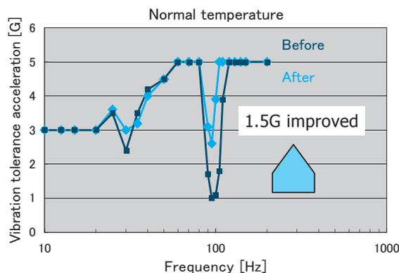
Fig.11 Rolling Correction Circuit Effect
