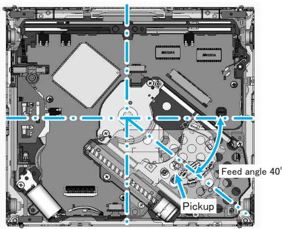
Fig.4 Pickup Layout on BD-01
