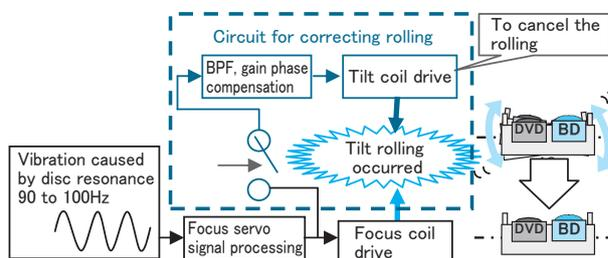
Fig.10 Block Diagram of Rolling Correction Circuit
