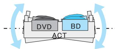
Fig.9 Rolling of TILT Actuator
