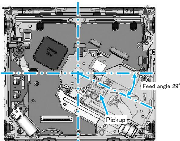
Fig.3 Pickup Layout on DV-05
