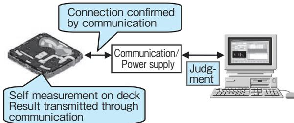
Fig.13 Simplified Process with Self-Check
