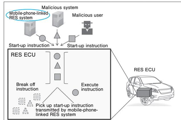
Fig.6 Prevention of Unauthorized Access
