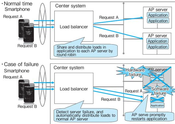
Fig.8 Structure of Fail-Safe
