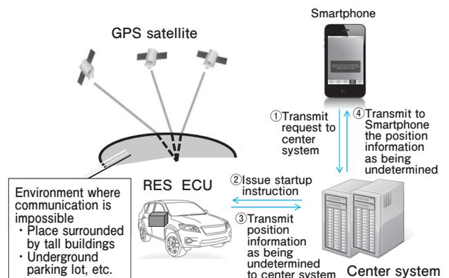
Fig.11 Prevention of Transmitting Erroneous Position Information
