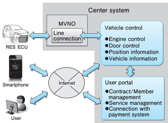
Fig.1 Center System Configuration of Mobile-Phone-Linked RES
