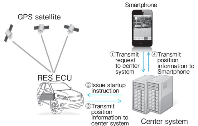
Fig.10 Method for Executing Carfinder Function
