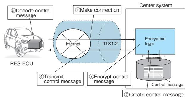
Fig.7 Flow of Processing for Encrypting Control Message
