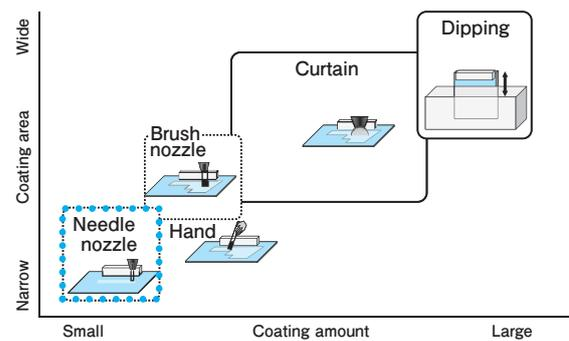
Fig.7 Types of coating method
