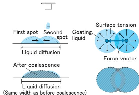
Fig.13 Liquid diffusion by multi-point coating
