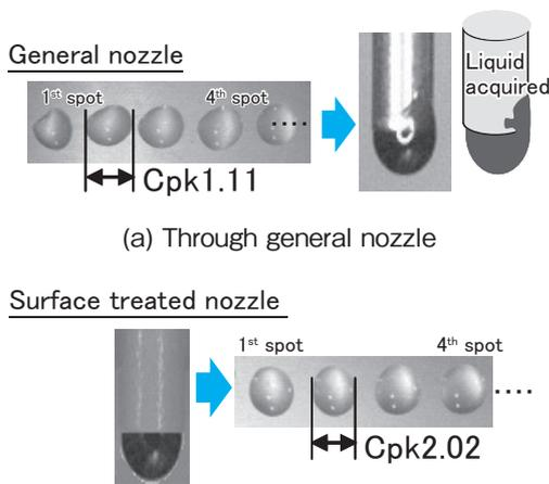
Fig.10 Coating through nozzle
