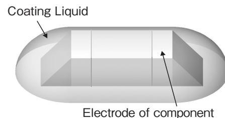
Fig.4 Typical coating pattern
