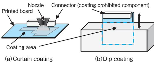
Fig.5 Types of coating method
