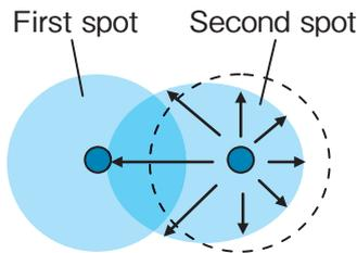
Fig.14 Image of method for controlling liquid diffusion
