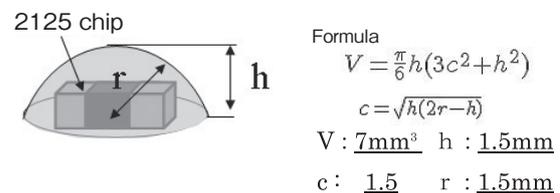
Fig.8 Coating amount calculation
