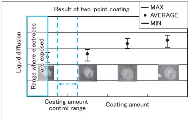
Fig.15 Coating amount control range
