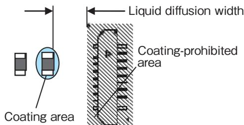
Fig.9 Target width of liquid diffusion
