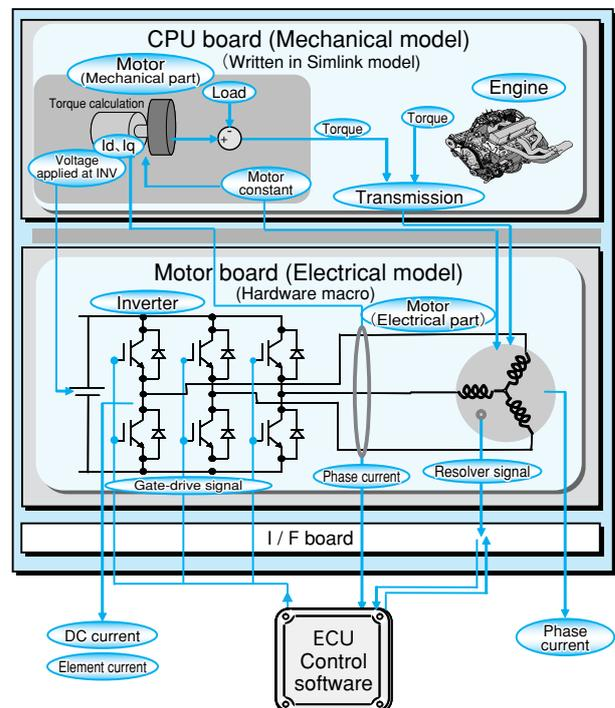
Fig.2 Motor Simulation
