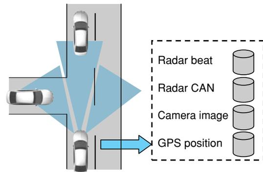
Fig.5 Measurement Data for Millimeter-Wave Radar
