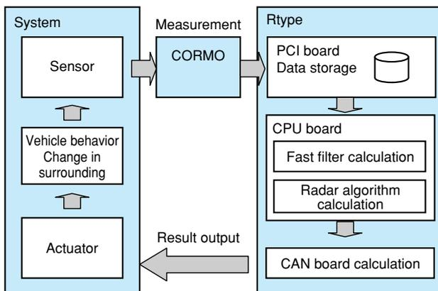
Fig.9 CORMO and Rtype Configuration Diagram
