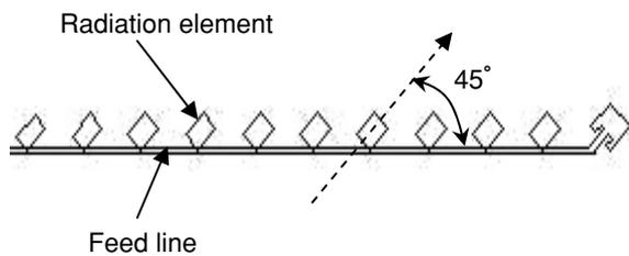
(a) Structure of feed line and radiation element
