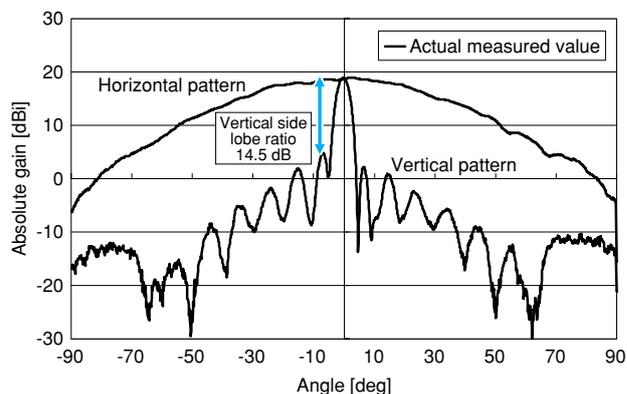
Fig.6 Evaluation Result of Antenna Pattern
