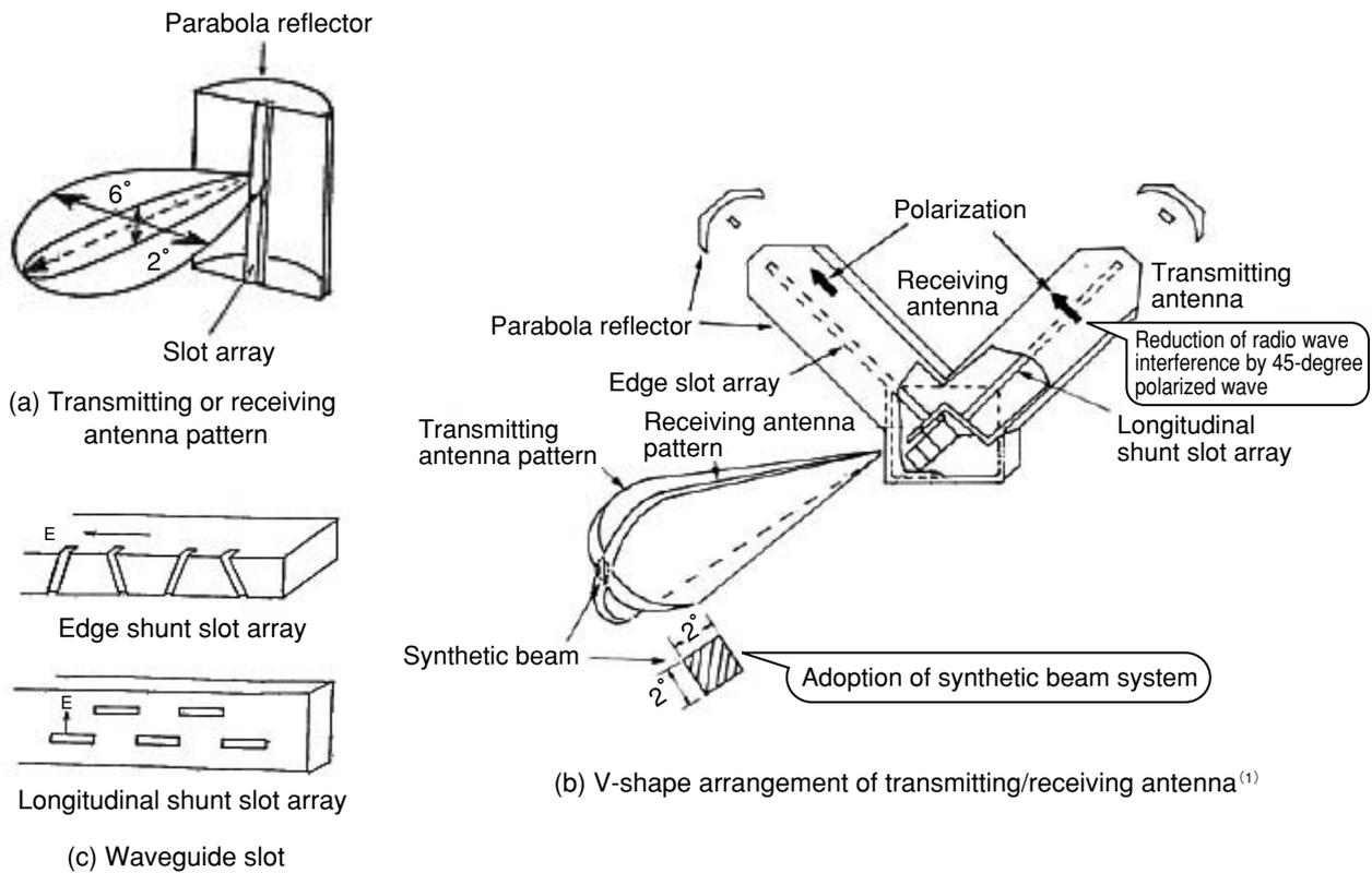
Fig.2 Structure of Waveguide Slot Antenna<sup>(1)</sup>
