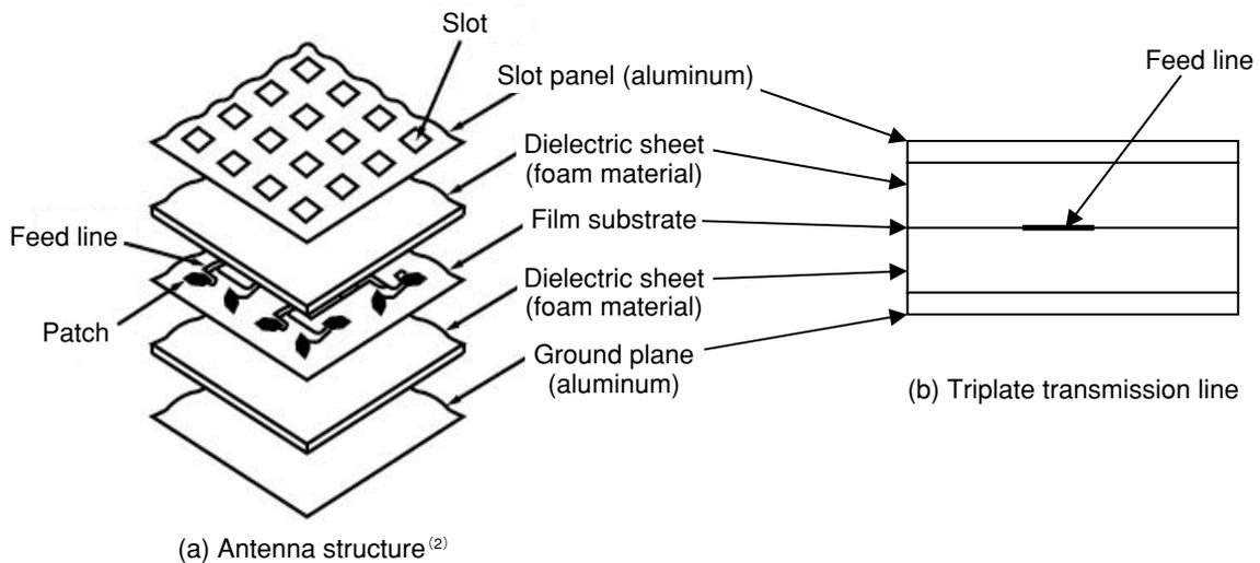
Fig.3 Structure of Triplate Antenna
