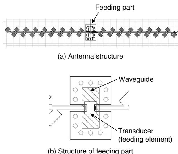
Fig.5 Structure of Center-fed Microstrip Antenna and its Feeding Point
