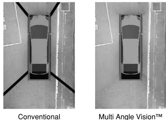
Fig.9 Examples of Borderlines between Camera Images
