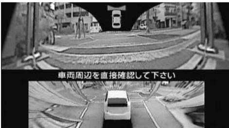
Fig.4 Image Used for Check at Intersection with Poor Visibility
