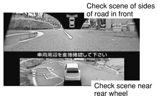
Fig.14 Images Used for Turning Left at Intersection with Poor Visibility
