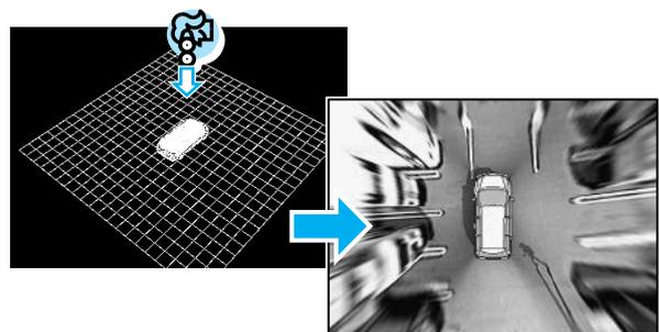
Fig.7 Image Example Projected on 2-D Model
