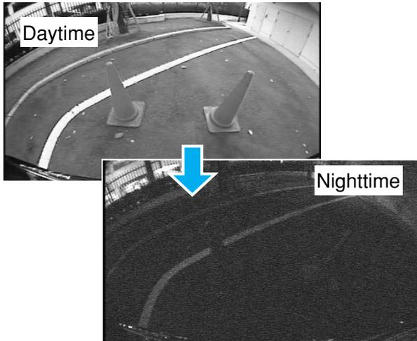
Fig.1 Difference in Camera Image Brightness between in Daytime and in Nighttime
