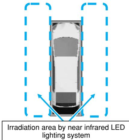
Fig.11 Irradiation Area by Near Infrared LED Lighting of This System
