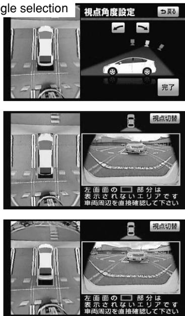
Fig.15 Images at Different Viewing Angles
