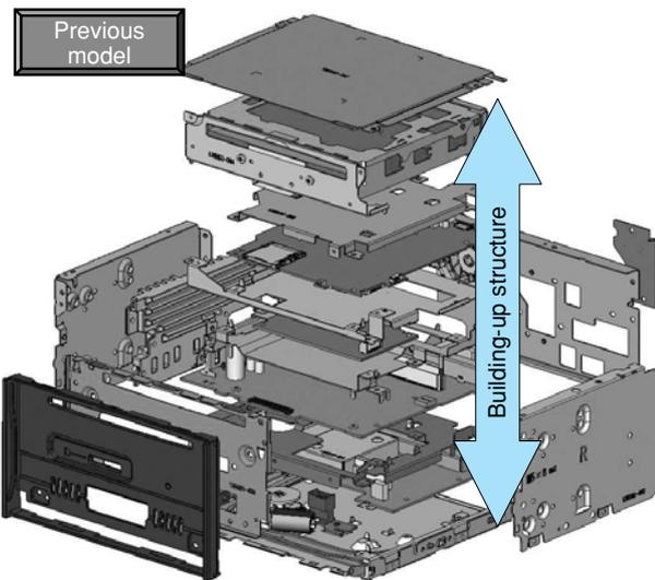
Fig.12 Exploded Diagram of Current AVN Lite
