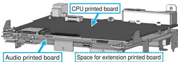
Fig.13 Printed Wiring Board ASSY
