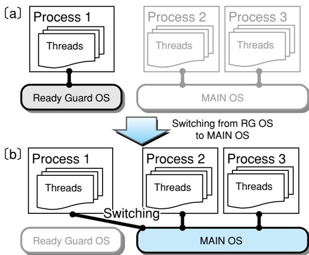
Fig.21 Structure of High-speed Start-up
