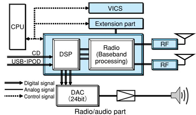
Fig.8 Block Configuration of Radio/Audio
