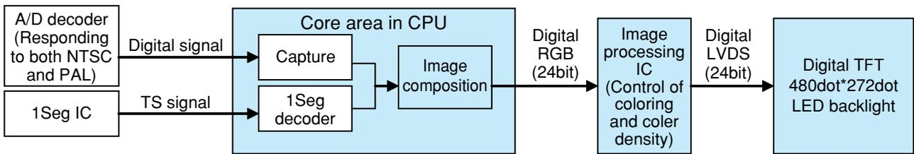
Fig.5 Block Configuration of Video
