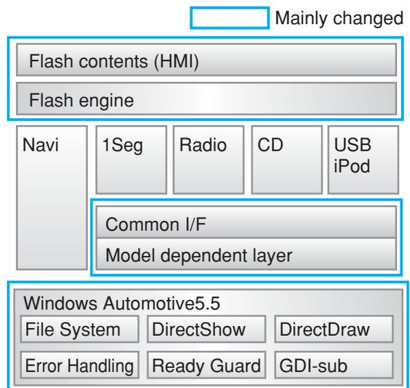
Fig.18 Software Configuration and Main Changed Points
