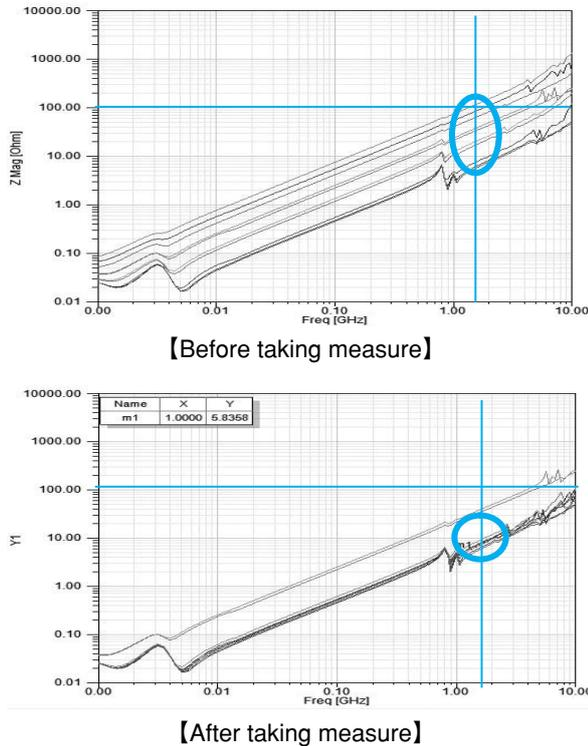
Fig.9 Power Source Impedance
