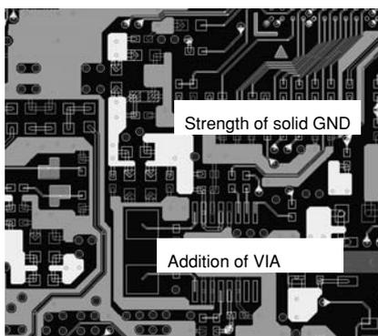
Fig.10 Example of Pattern Reflection
