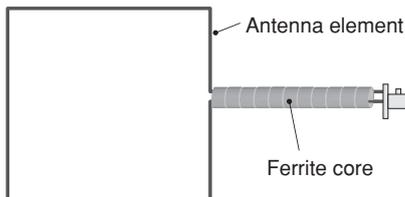
Fig.5 Antenna Structure
