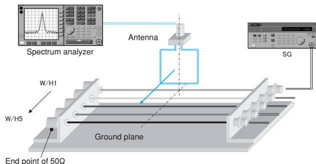
Fig.4 Measurement Environment
