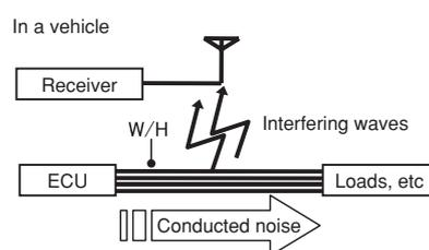
Fig.1 Mechanism of Noise Interference
