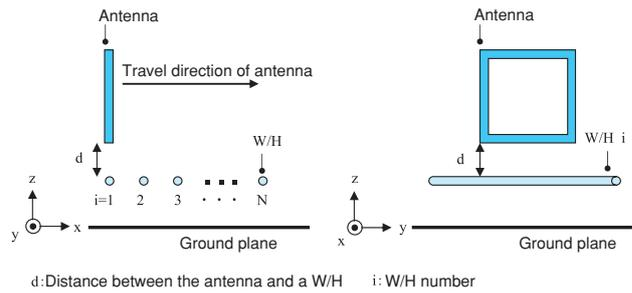
Fig.3 Noise Detection and Measurement System
