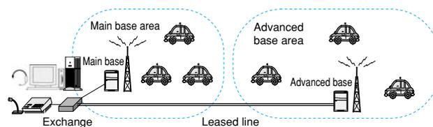
Fig.7 Composition Example of Two Base Stations
