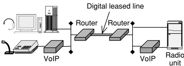
Fig.8 Analog Connection and IP Connection
