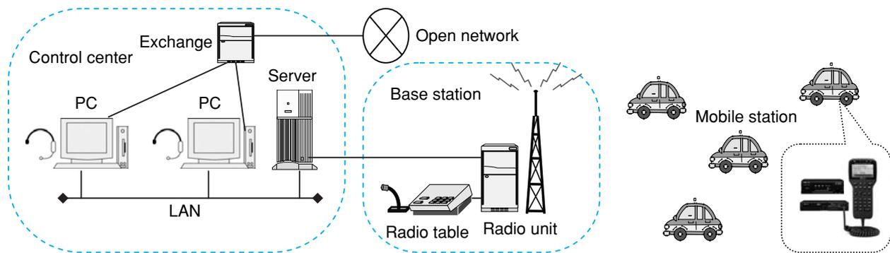
Fig.2 Image Drawing of AVM System Components
