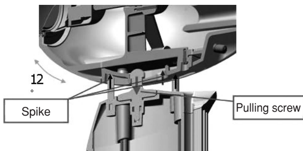
Fig.17 Angle Adjustment Structure of TD712zMK2
