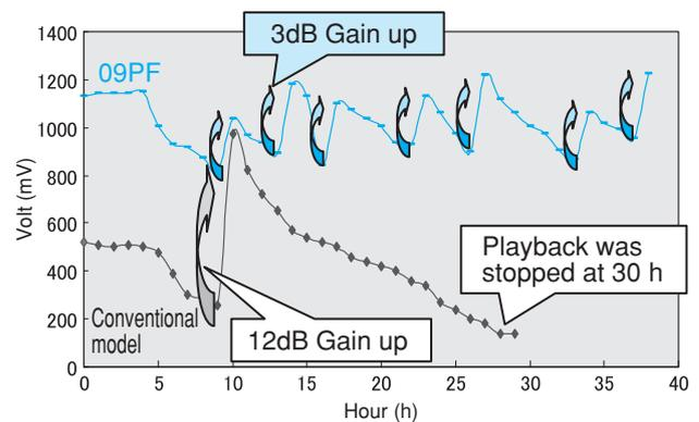
Fig.14 Comparative Efficacy with Dust Test
