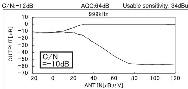
Fig.7 One Signal Characteristic of Conventional Model (07PF) with Antenna Amplifier for Short Pole Combined
