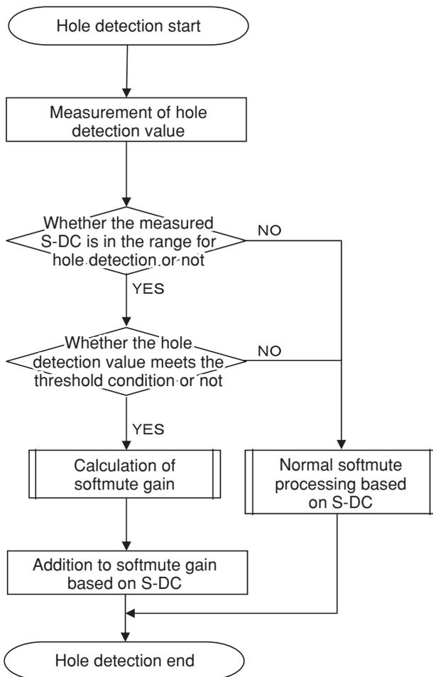
Fig.11 Soft-mute Processing following Hole Detection
