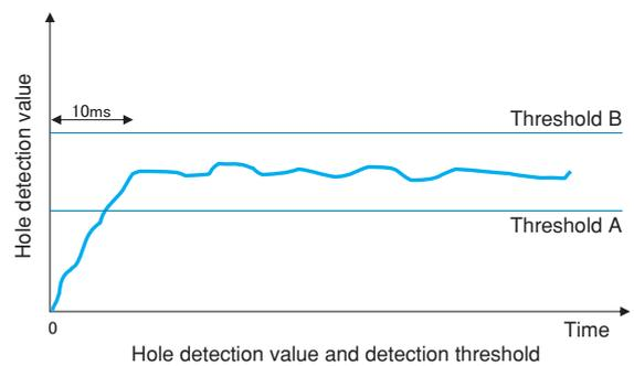
Fig.10 Relation between Hole Detection Amount and Threshold
