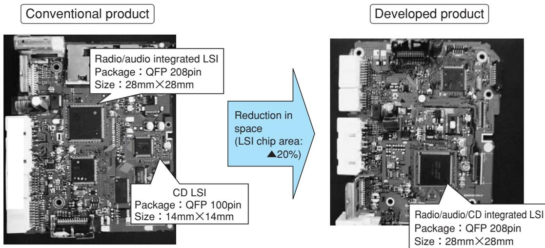
Fig.15 Comparison of Main Printed Boards in CD-tuners Equipped with Developed Product and Conventional Product
