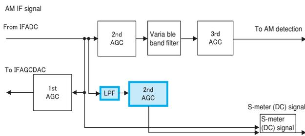
Fig.6 Block Circuit of DC Part S-meter
