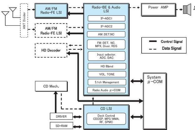
Fig.2 System Block Diagram of Conventional Product (07 model)
