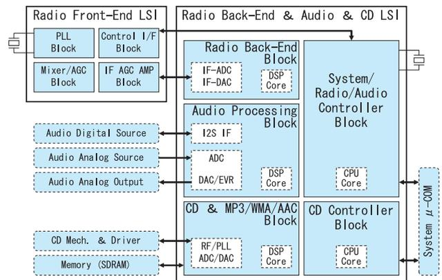
Fig.4 Device Configuration Diagram
