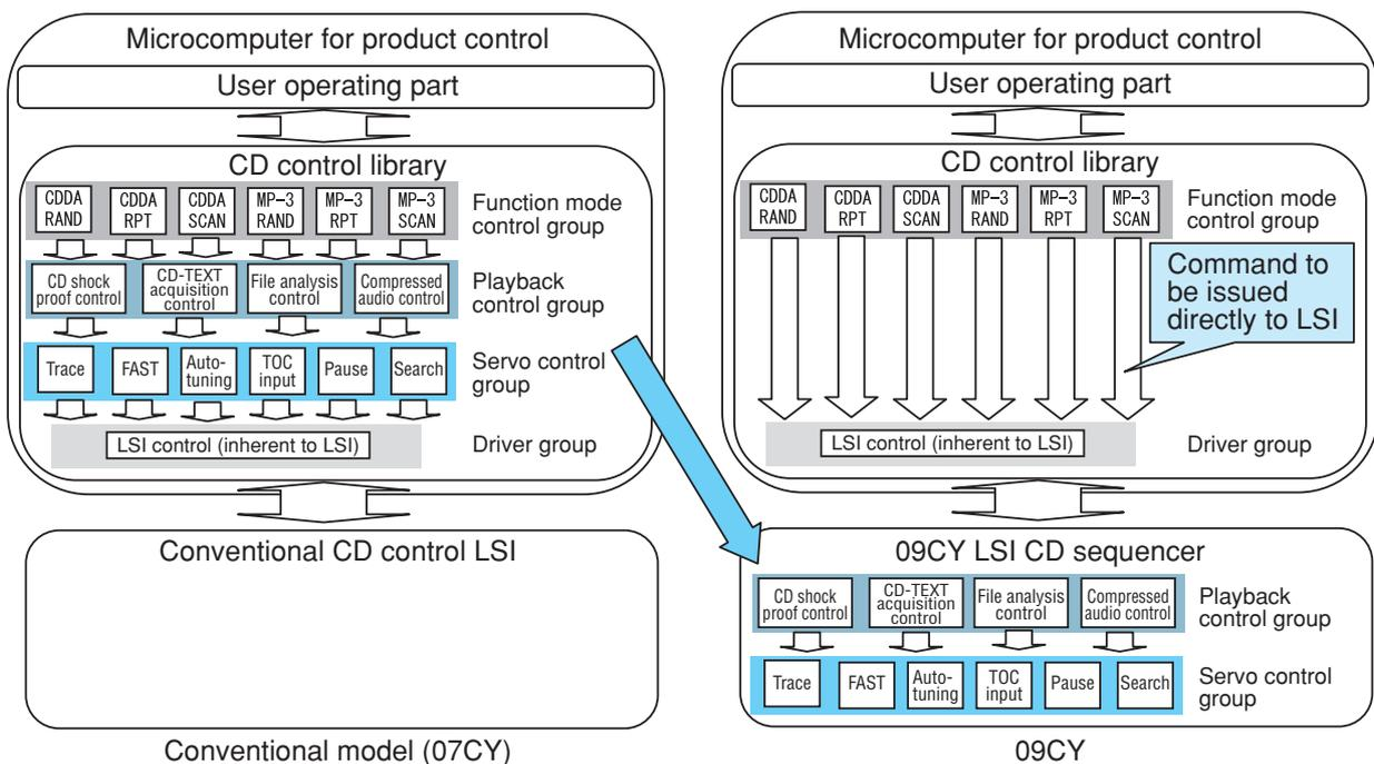
Fig.12 Block Diagram of CD Control Firmware
