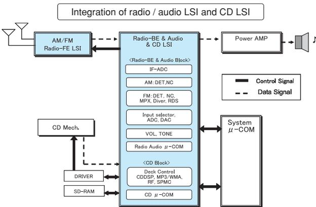
Fig.3 System Block Diagram of Developed Product (09 model)
