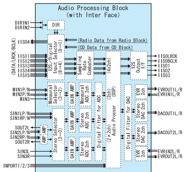
Fig.5 Diagram of Audio Processing Block
