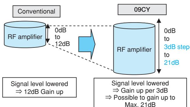
Fig.13 Variable Amount Expansion of Control Gain
