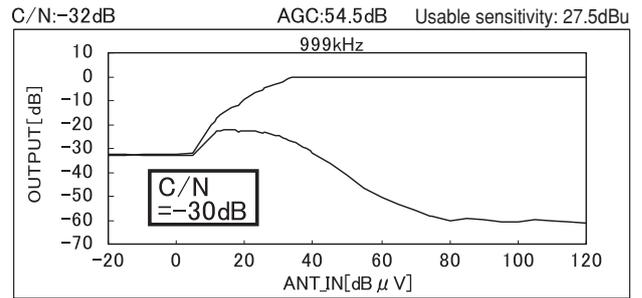
Fig.8 One Signal Characteristic of New Model (09PF) with Antenna Amplifier for Short Pole Combined
