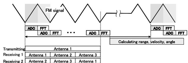
Fig.11 Control Timing
