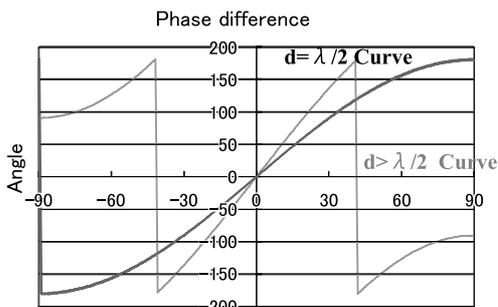
Fig.6 Angle vs. Phase Difference
