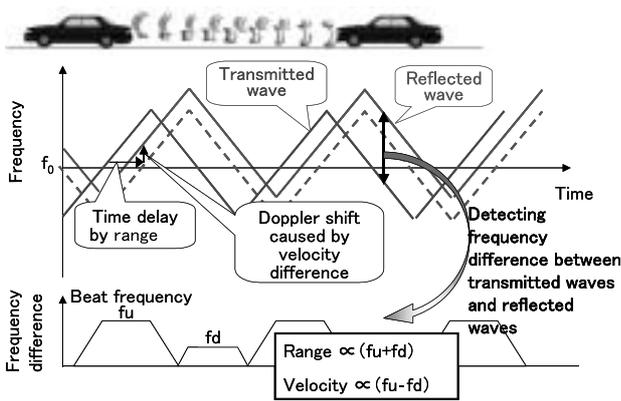
Fig.9 Principle of FM-CW Radar
