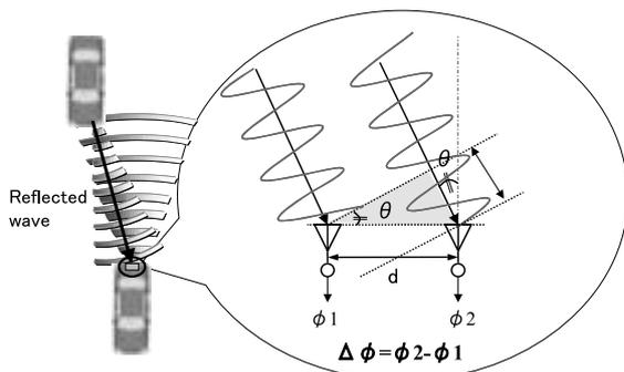
Fig.5 Principle of Monopulse System
