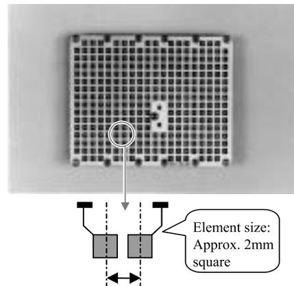
Fig.7 Image of Planar Array Antenna
