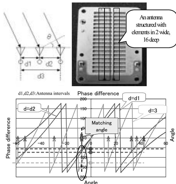
Fig.8 Relation of 3ch Monopulse Antenna and "Angle vs. Phase Difference"
