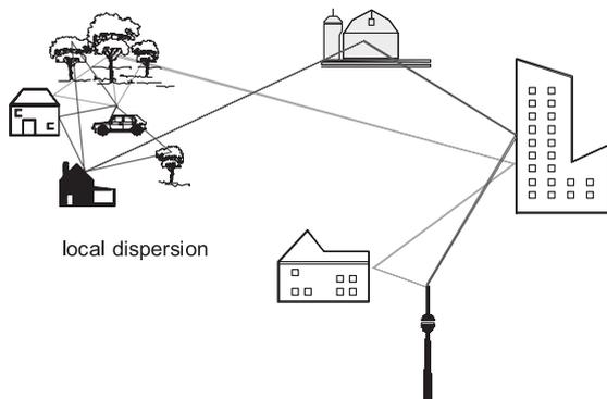
Fig.1 Multipath propagation
