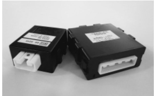
Fig.1 Gateway ECU (left) and Translate ECU (right) of FUJITSU TEN
