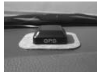
Fig.2 GPS patch antenna for car navigation
