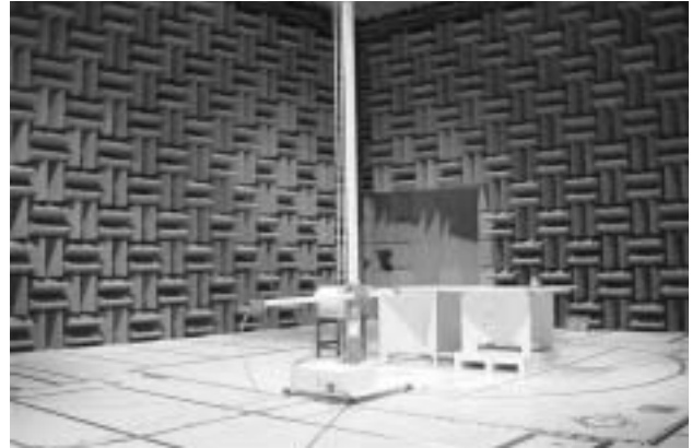
Fig.2 No. 1 Radio wave semi-anechoic chamber (10m method)
