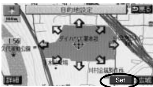
Fig.15 Procedure for setting destination with i-NaviLink
