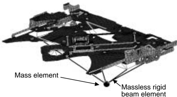
Fig.19 Model for analysis using large mass method
