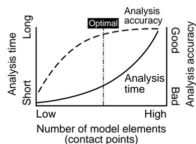
Fig.4 Graph plotting number of elements versus analysis time
