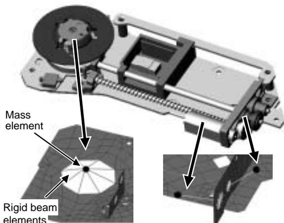
Fig.12 Mass element model
