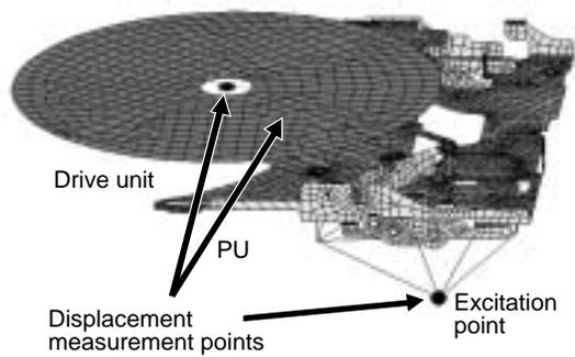
Fig.22 Displacement measurement positions
