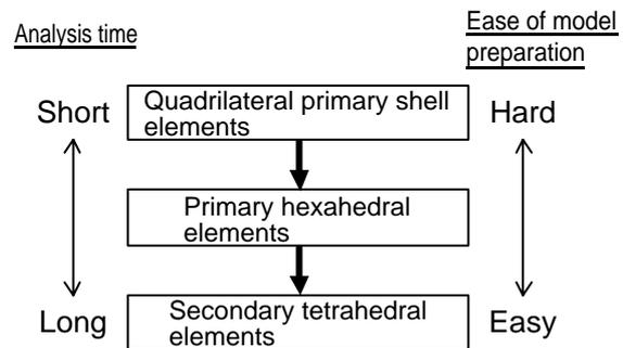
Fig.2 Procedure for element selection
