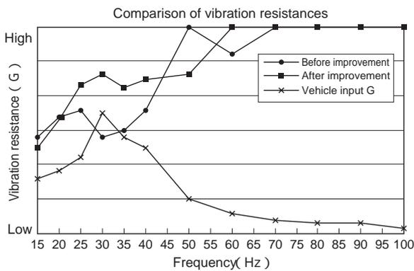
Fig.28 Vibration resistance performance graph for item with improved vibration resistance construction
