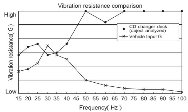
Fig.21 Vibration resistance performance graph
