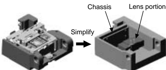
Fig.7 Simplified 3-D CAD model of PU
