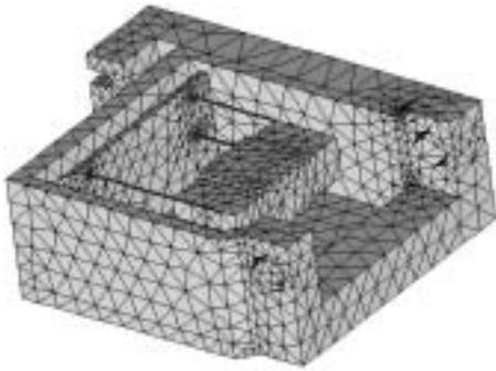
Fig.11 Mesh model of PU
