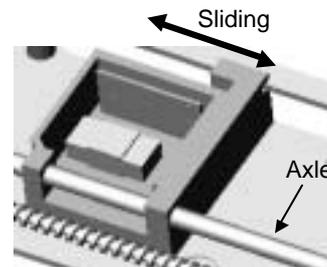
Fig.17 Sliding along axle
