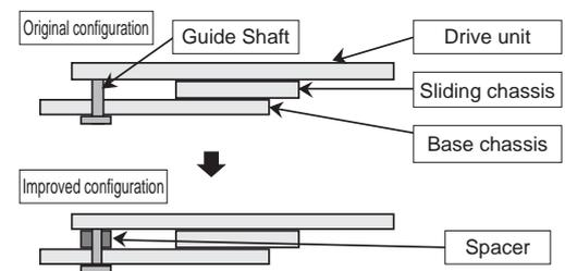
Fig.27 Vibration resistant construction proposal 2
