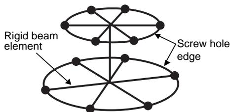
Fig.16 Joining of rigid beam elements
