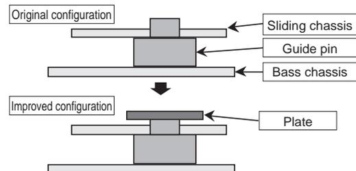
Fig.26 Vibration resistant construction proposal 1
