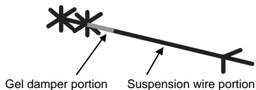
Fig.10 Suspension model
