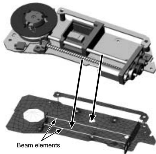
Fig.13 Axle beam element model
