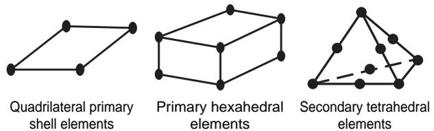
Fig.3 Element configurations
