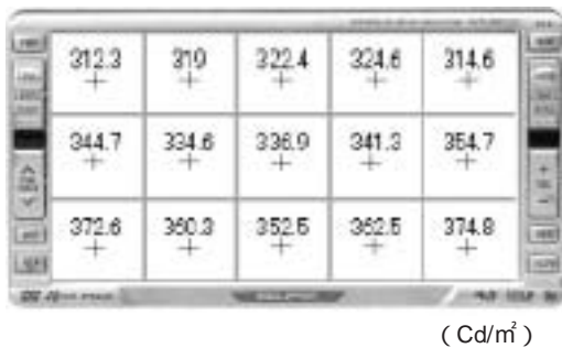
Fig.11 Screen brightness distribution at VGA display surface
