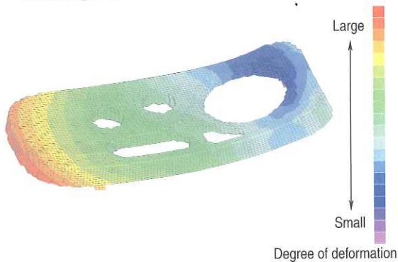
Fig. 4 Diagram of predicted warp and deformation
