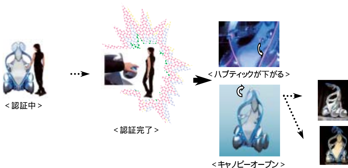
図-21 個人認証の手順 Fig.21 Procedure for individual identification
