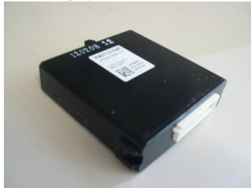
Keyless access upgrade ECU
